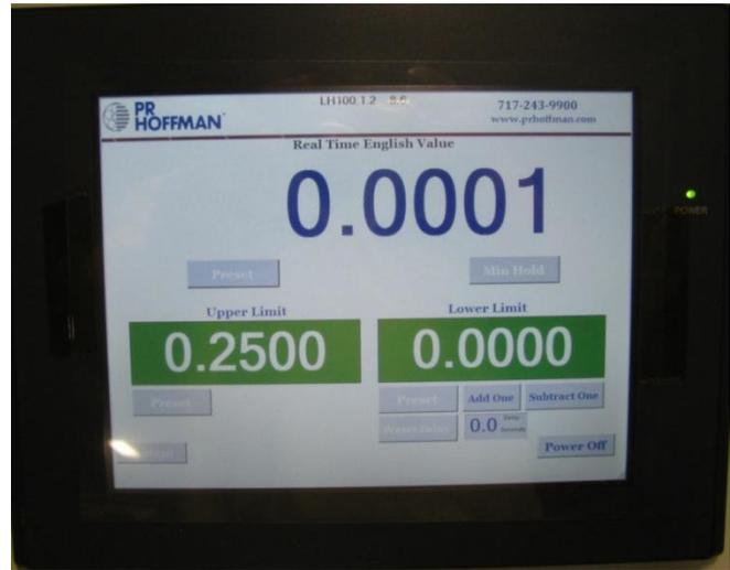
The operator presets the amount of material to be removed on the touch screen control in inches, microns or millimeters. The gauge device then shuts the machine off when this amount of material is removed. Typically, this gauge can be used to process parts to tolerances of  $\pm 0.0002$ " [5 microns] or better.
