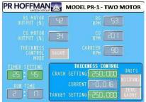
The dual motor PR-1 touch screen control is the same as the standard configuration, with the additional display of separate motor power outputs and the addition of a screen for selecting the pre-programmed carrier rotations for the high and low mode operation.
