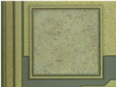
Figure 2: Aluminum bond pads showing corrosion after dicing
