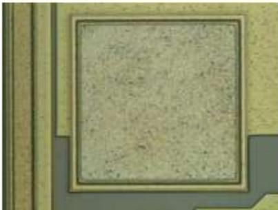
Figure 2: Aluminum bond pads showing corrosion after dicing
